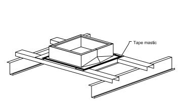
3) Apply tape mastic around the outside of curb flange.
